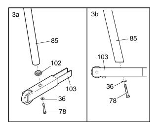
4. Slide the upper end of a Handrail (85) and then the Extension Leg (103) into the right Upright (82) as shown. (Note: It may be helpful to tip the Uprights [82] forward as you insert the Extension Leg. If necessary, tap the Extension Leg with a rubber mallet to fully insert it.)
